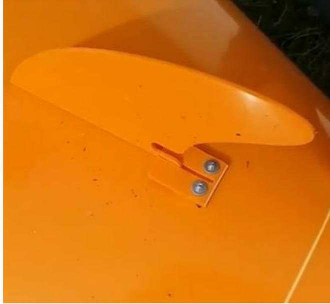
2) To fold back down for storage, lift the tab on the left side at the bottom of the fin so that the fin will fold back down underneath the positioning tabs.
