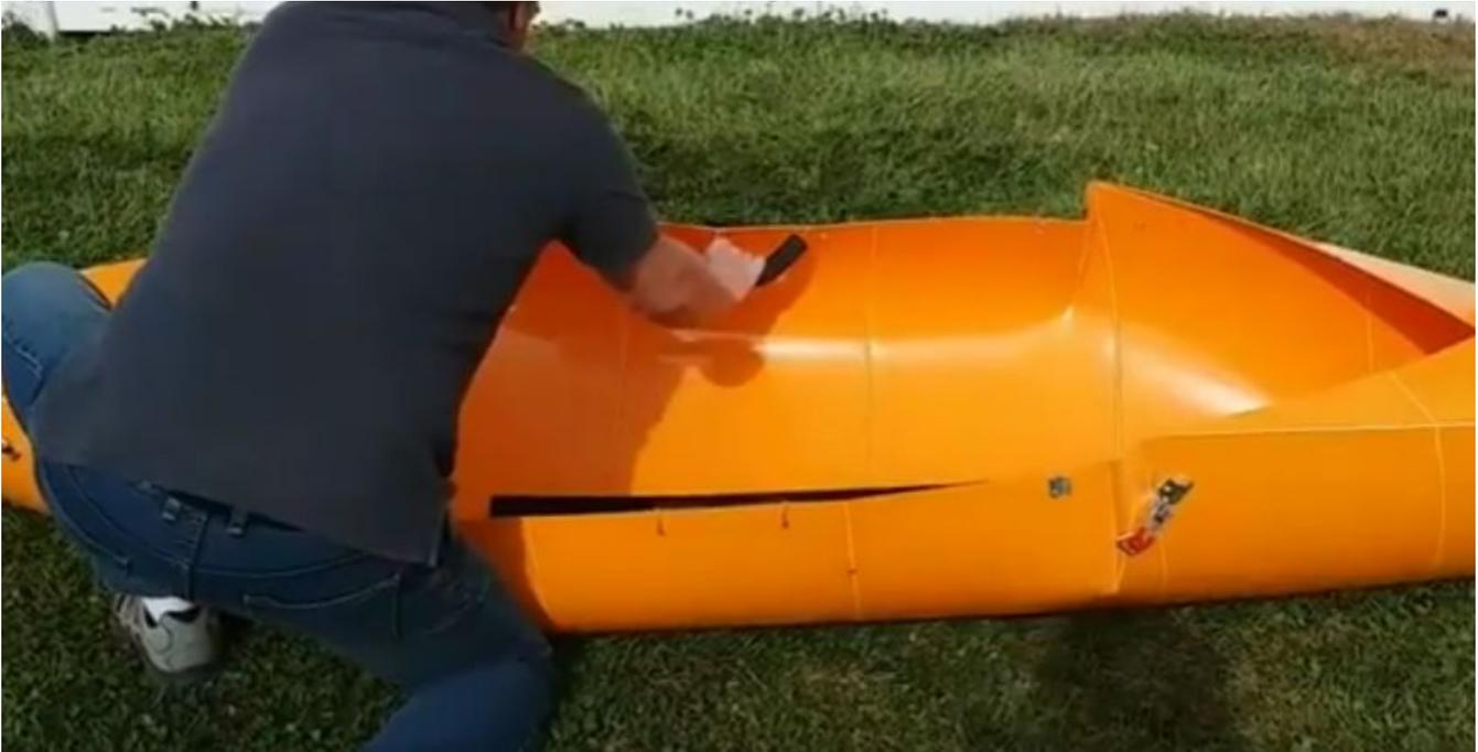
7) Move to the STERN side clamps and repeat the process. First one side then the other. The stern end will have swiveling clamps. This will ensure the canoe will fold in properly. Pull the handle towards you and down the same way you do with the bow end, while holding the clamps in the open position as well as swiveling them to align with the catch.
