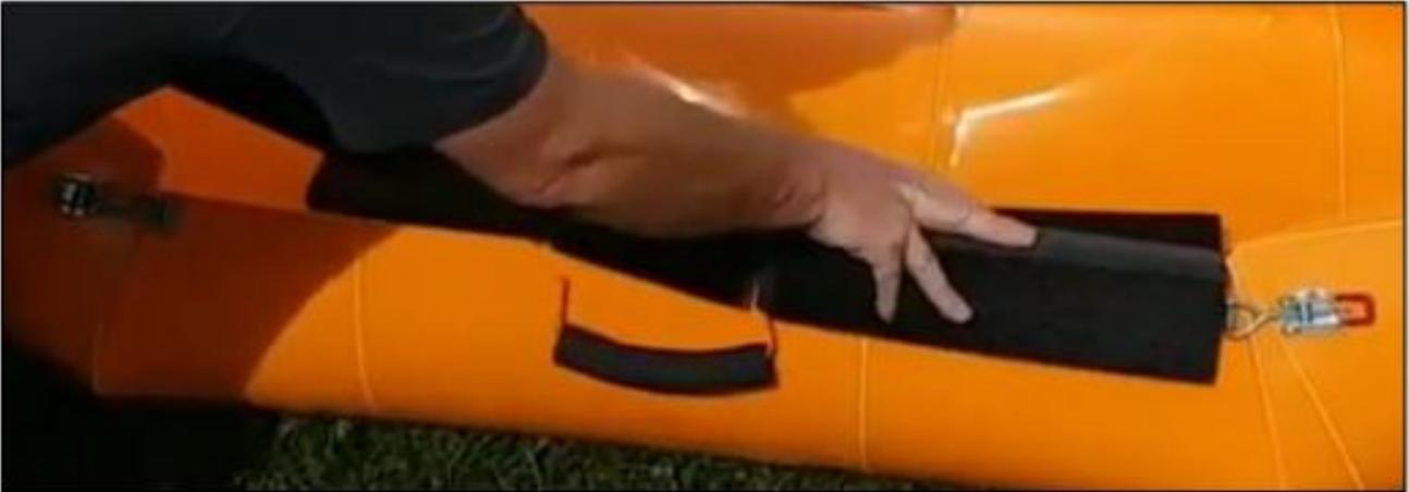
Once the foam rail is pushed fully down over the side pull the handle up with the paracord going through the grooves until the handle sits on top of the foam rail.
