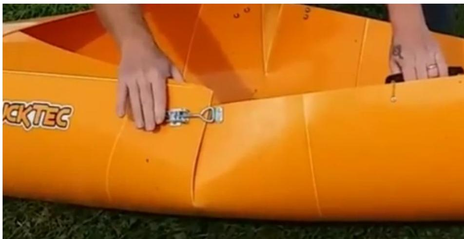
6) Move to the LEFT side of the Kayak to repeat the process with the clamp on the RIGHT side. Reaching across and pulling the handle in and down while holding the clamp in the open position and pushing in and down until they meet to catch. Close clamp.
