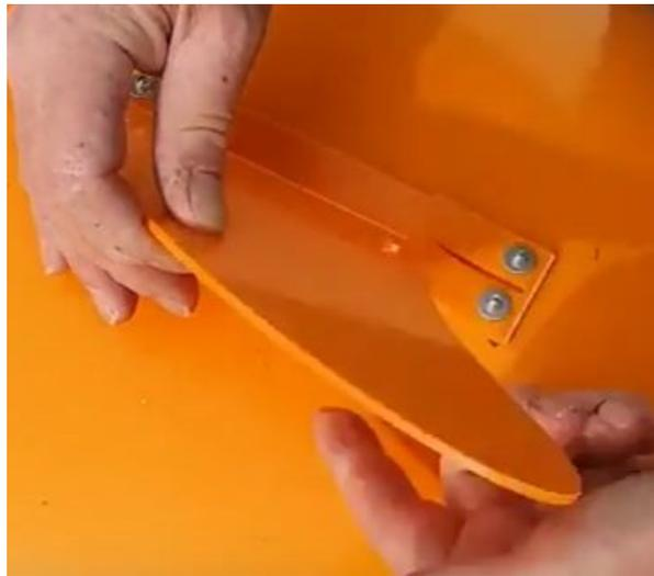
NOTES: Try to wait until you are ready to place the Kayak in the water before setting up the fin. Place the back end of the Kayak into the water with enough depth so that the fin does not hit bottom. If the fin does hit bottom or get bent out of position, it should ease back on its own. The plastic is flexible so you can always bend back into shape and lift the positioning tabs to hold better.
