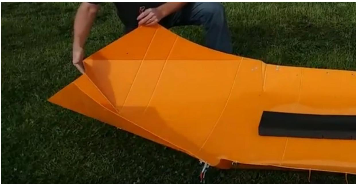
3) From the RIGHT side of the sheet (with the clamp in the open position) bring the clamp end flap up and over while pulling-in the opposite end flap (using your body as a brace) and latch the clamp onto the “catch” located part way down the bow side. Secure and close clamp.
